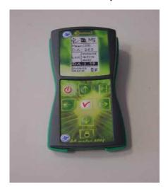
In kiwi the optimal harvest time is a crucial issue, since fruit shelf-life potential and quality are closely related to the ripening stage at harvest. The Kiwi Meter is a very promising tool both for practical and scientific applications, since it allows to monitor on-tree fruit ripening (as well on the same fruit), to establish accurately the optimal harvest time and it can be used in cool store to establish maturity changes as well.
